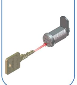
**Step 2:** Rotate the core 90° past the normal function of the lock and in the same direction.
