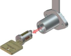
Lock Housing Ready for Core Insertion.
