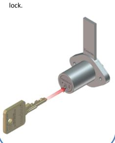
**Step 2:** Rotate the core 90° past the normal function of the lock and in the same direction.
