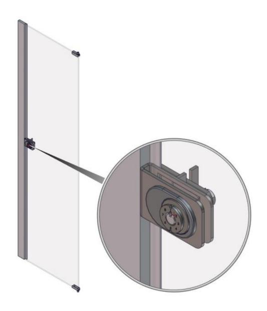
1) First determine the distance from the locking edge of the glass to the center of the installation hole. Using this distance note the orientation of the dress plate on the diagrams to the right.
